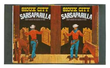
For many years, the soldered method was the mainstay. The areas outside of the decoration, right and left, were bare tinplate. The decorated flat sheets were slit into body blanks (above) and the cans were formed and soldered on the bodymaker. Ends were then seamed on both ends of the can.
